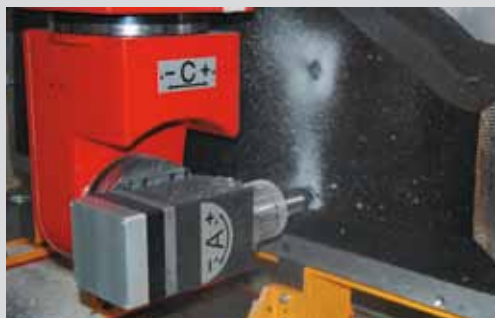
Aeronautic part trimming Material: Carbon fibre
