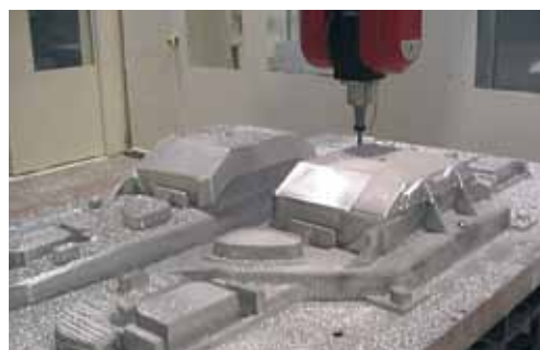
Aluminium mold Material: Aluminium
