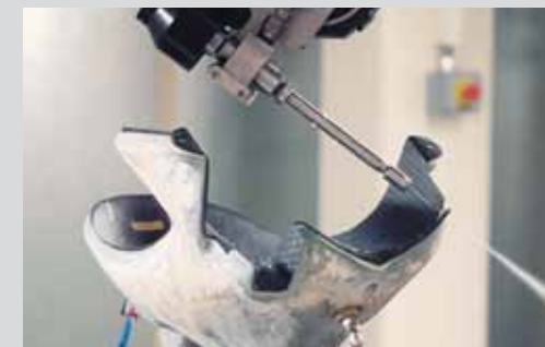
Motorbike fender trimming Material: Carbon fibre
