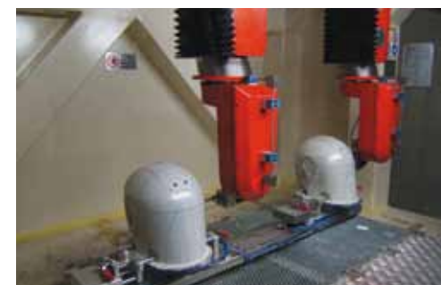
Simultaneous cutting of two helmets Material: Glass fibre
