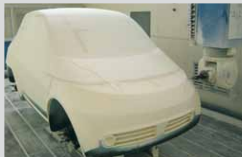
Car mold milling. Material: Resin
